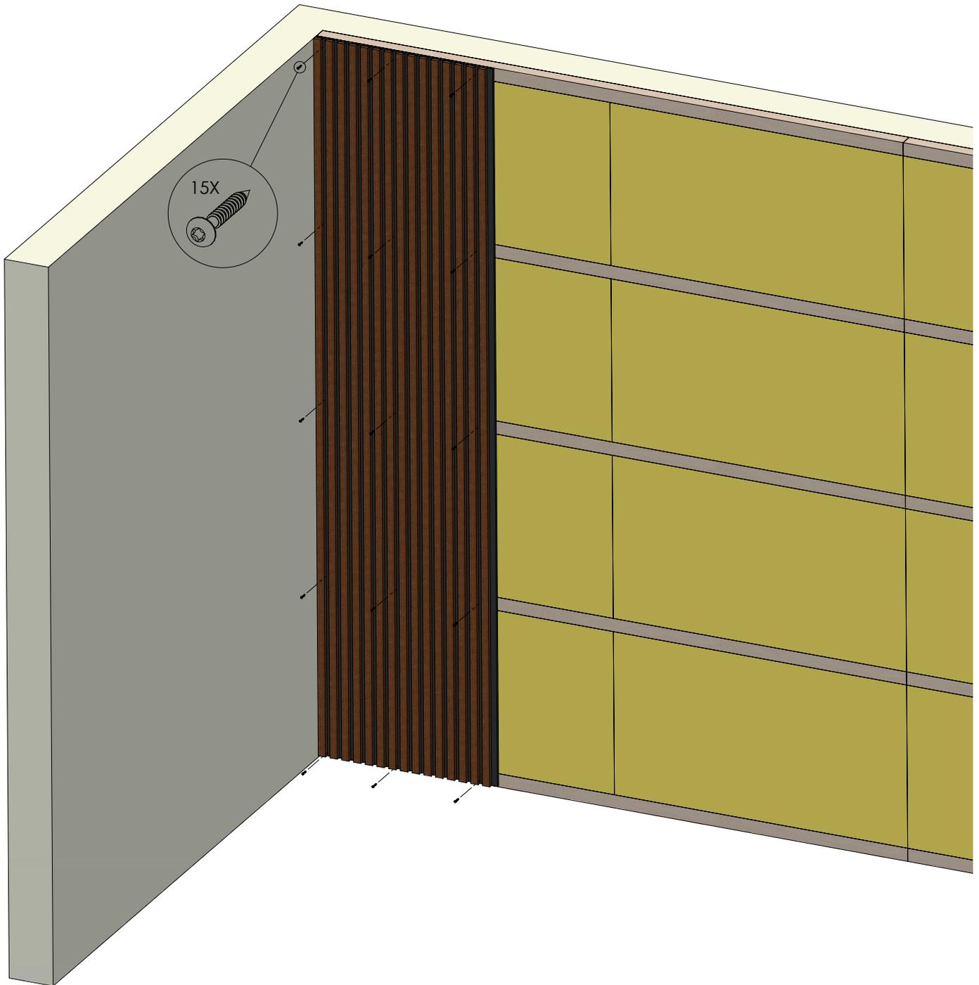
There are different ways to mount Ribbon-Wood. You can screw or glue the panels on existing walls / ceilings. If you want even better acoustics in the room, you can unbolt 45x45mm wooden rule and set insulation (45mm) in between, then you achieve sound class A.
